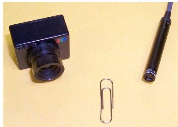
Figure 2. Two miniature CCD cameras used in this work.
