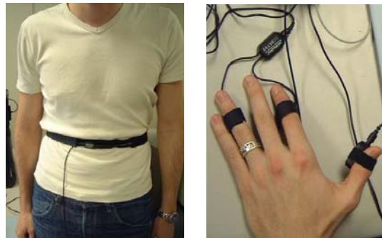
Figure 1 The sensors used to measure respiration (abdomen), skin conductance (fingers of one hand), and blood volume pulse (thumb of one hand)
