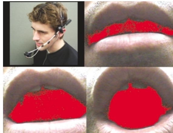
Figure 1. The head mounted video camera with views of the vowels [i], [a], and [o]. The segmented area is shown in red.
